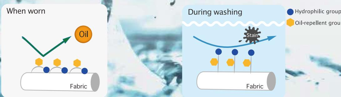
\*Due to the flip-flop phenomenon, oil-repellent groups and water-repellent groups repel dirt in the air, and hydrophilic groups release stains in water.
