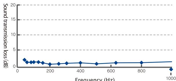
\*The sound insulation property is measured by the sound transmission loss (acoustic tube measuring method ASTM E2611-09).
