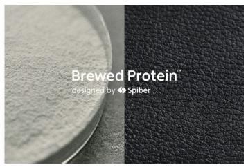
Brewed Protein™ materials are the protein fibers, films, and other types of polymer materials manufactured using Spiber's proprietary microbial fermentation (brewing) process. Made from plant-derived sugars as primary raw ingredients, Brewed Protein™ materials offer a solution to address increasing market demand for animal-free, plastic-free alternatives to conventional materials. Spiber has
